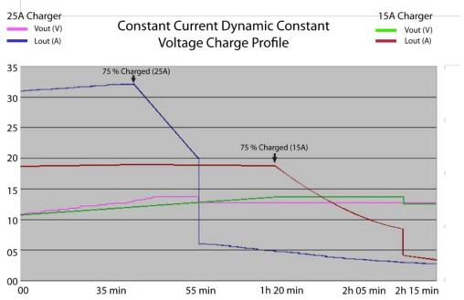
This graph shows Here is the constant current dynamic constant voltage charge profile (stays in boost for 50% of the time it took to reach the boost voltage)
