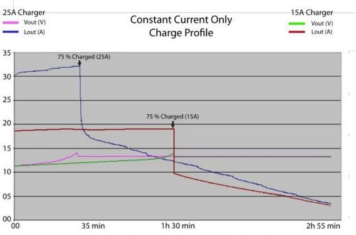
This graph shows the constant current only output regime charge profile (comes out of boost mode when the boost voltage is reached)
